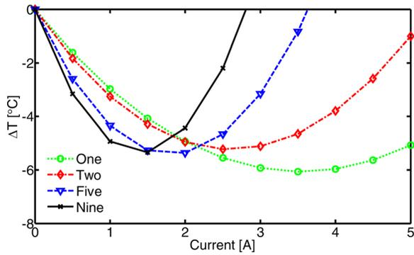
**Fig. 3** Temperature change at the center hot spot ( $\Delta T$ ) for various configurations of active hot spots and TECs: (1) Only center hot spot active, (2) Hot spots 5 and 6 active, (3) Hot spots 2, 4, 5, 6, and 8 active, (4) All nine hot spots active
