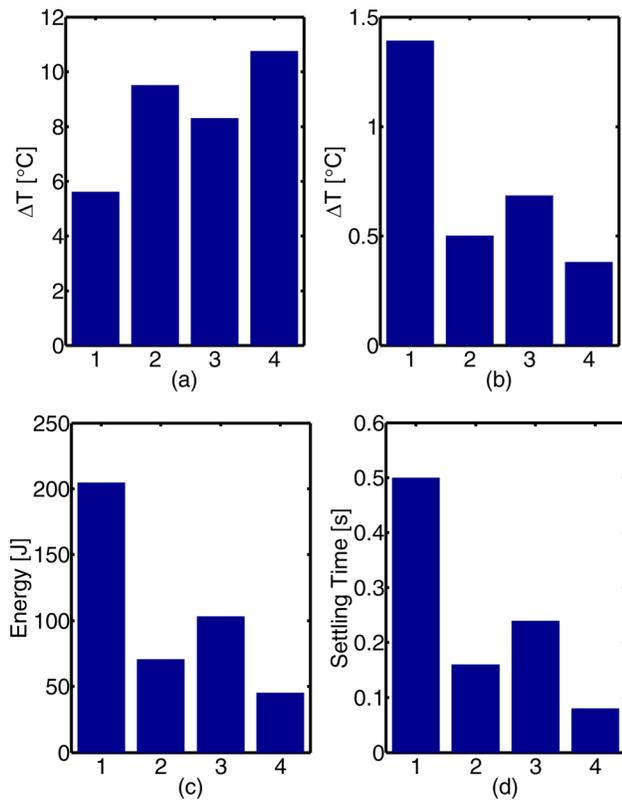
**Fig. 10 Comparison of the four pulses: (1) Constant, (2) Linear, (3) Square Root and (4) Parabolic using four parameters important to select a pulse: (a) Difference between maximum temperature and threshold temperature ( $\sim 102^\circ\text{C}$ ), (b) Temperature overshoot after pulse is turned off, (c) Total energy expended during pulsed operation and (d) Settling time for temperature within  $0.5^\circ\text{C}$  of steady-state**
