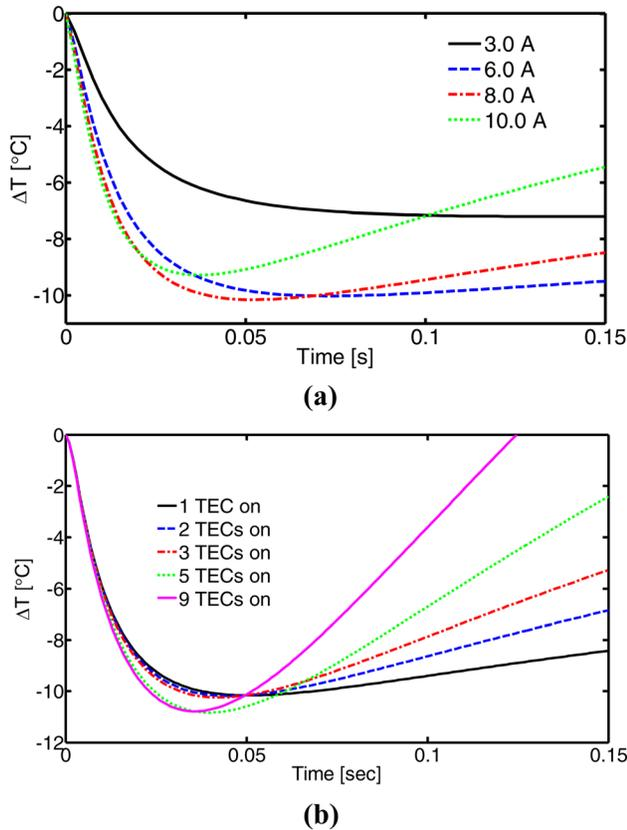
**Fig. 6 (a) Transient analysis of a single hot spot; TEC turned on with 3.0 A, 6.0 A, 8.0 A, and 10.0 A current; (b) Transient analysis with 8.0 A current for various number of hotspots and active TECs**
