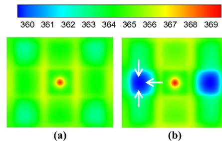
**Fig. 5** Temperature contours in a horizontal cross-section of chip at  $10 \mu\text{m}$  below the chip-TIM interface when only center hotspot is active. (a) center TEC turned on at 2 amperes, and (b) center and two adjacent TECs turned on at 2 amperes; arrow shows heat flow direction due to the active TEC at left side.
