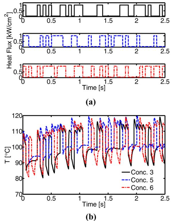
**Fig. 11 (a) Random cycling of hot spots 3, 5 and 6, respectively; (b) Transient temperature at hot spots when TECs turned on with square root pulse at hot spot temperature  $> 102^\circ\text{C}$  during random cycling of hot spots**
