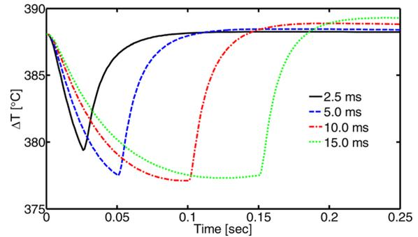
**Fig. 8** Hot spot 5 turned on with a high heat flux of  $1000 \text{ W/cm}^2$  and allowed to reach steady-state; TEC turns on with square root pulse of various periods: 2.5 ms, 5.0 ms, 10.0 ms, 15.0 ms
