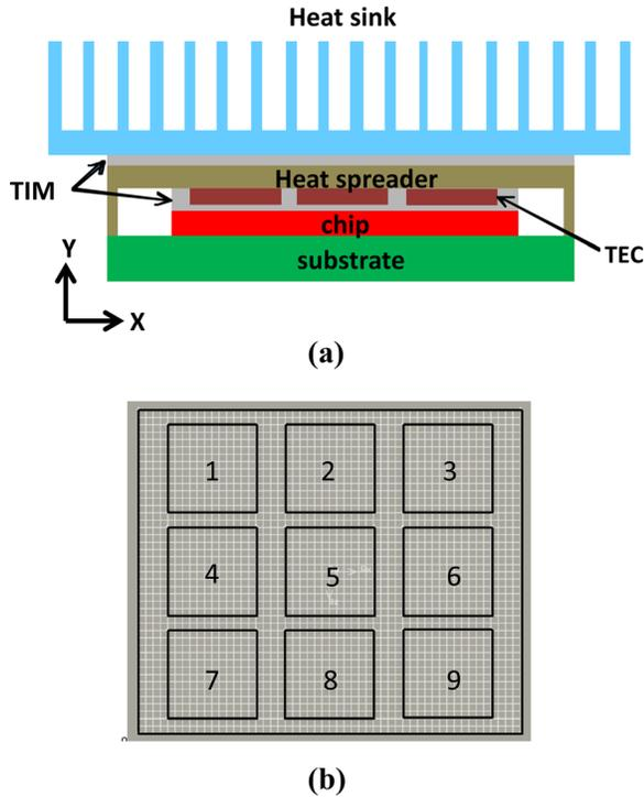
**Fig. 1** (a) Schematic of an electronic package. Heat spreader, thermal interface material (TIM), chip, substrate and thermoelectric coolers (TECs) are shown. (b) Layout of nine TECs and the associated mesh in a 2D cross-section.
