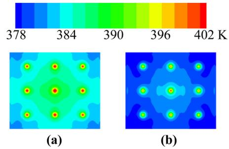
**Fig. 2** (a) Temperature contours on the bottom surface of the chip with no TECs turned on. High heat flux ( $1000 \text{ W/cm}^2$ ) sources are located at nine symmetrical points of area  $500 \times 500 \mu\text{m}^2$  which generate hot-spots. The rest of the surface has a uniform heat flux of  $43 \text{ W/cm}^2$ . (b) Temperature contours on the bottom surface of the chip with TECs turned on at 1.5 amperes.
