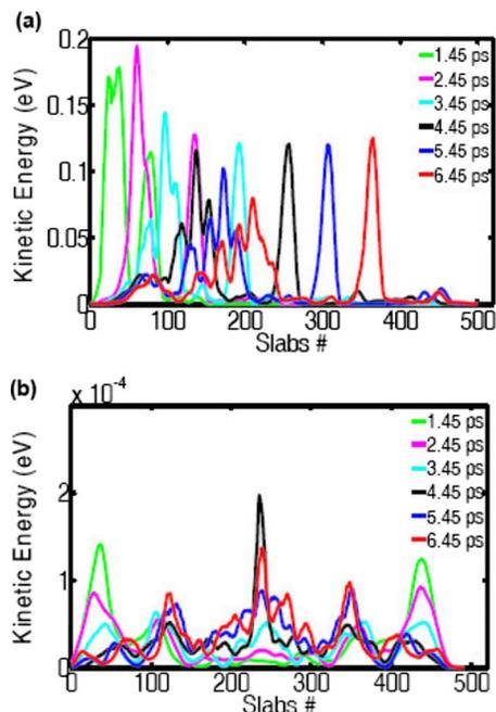
FIG. 6. (Color online) (a) The location and shape of the heat pulse at different time instants along the first CNT for (10,0) chirality. The pulse generation started at  $t=0.0$  ps. (b) The location and shape of the heat pulse at different time instants in the second CNT, also of the same chirality.
