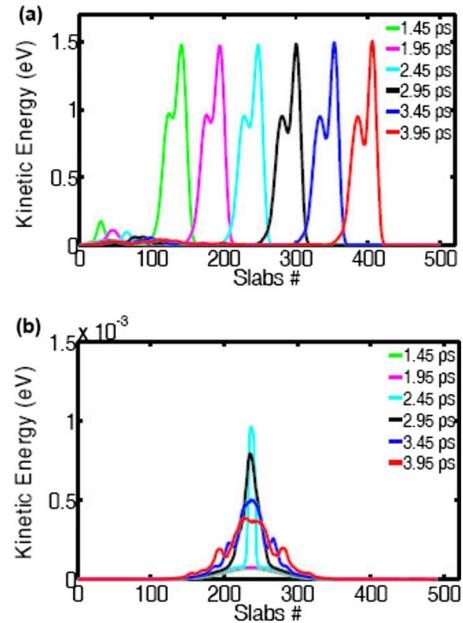
FIG. 4. (Color online) (a) The location and shape of the heat pulse at different time instants along the first CNT for (7,0) chirality. The pulse generation started at  $t=0.0$  ps. (b) The location and shape of the heat pulse at different time instants in the second CNT, also of the same chirality.
