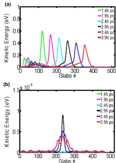
FIG. 5. (Color online) (a) The location and shape of the heat pulse at different time instants along the first CNT for (8,0) chirality. The pulse generation started at  $t=0.0$  ps. (b) The location and shape of the heat pulse at different time instants in the second CNT, also of the same chirality.
