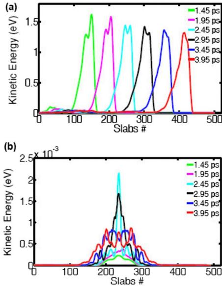
FIG. 3. (Color online) (a) The location and shape of the heat pulse at different time instants along the first CNT for (5,0) chirality. The pulse generation started at  $t=0.0$  ps. (b) The location and shape of the heat pulse at different time instants in the second CNT, also of the same chirality.
