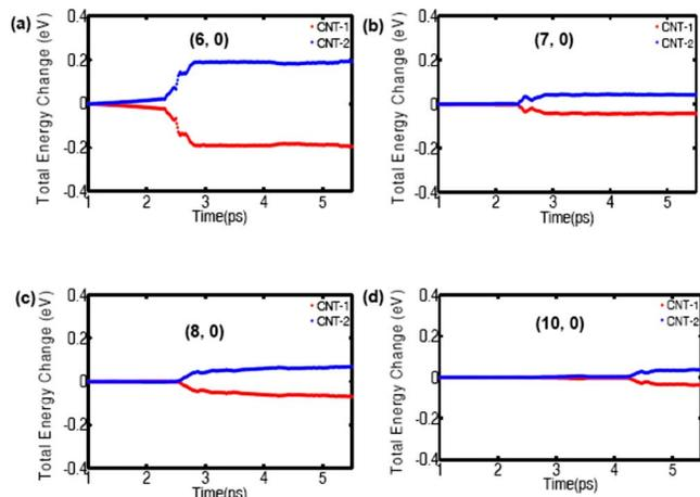
FIG. 7. (Color online) Change in the total energy of CNTs as a function of time with reference total energy corresponding to  $t=1$  ps. At  $t=1$  ps, the pulse generated in CNT-1 starts to propagate toward the contact region of the two CNTs. Here, CNT-1 corresponds to the CNT in which the pulse is generated; CNT-2 is located in a crossed configuration with respect to CNT-1. The chiralities of the CNTs are (a) (6,0) (b) (7,0) (c) (8,0), and (d) (10,0).
