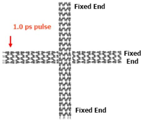
FIG. 1. (Color online) Schematic of two CNTs in a crossed configuration. A 1.0 ps pulse is generated from one end of the first tube, while atoms at the other end are kept fixed. The two ends of the other tube are kept fixed. The chiralities of the two tubes are the same.
